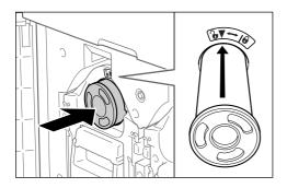
Align the arrow on the Ink Cartridge to the mark on the Print Drum (Cylinder) unit, and insert until it stops.
