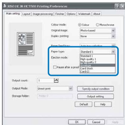
**11** Select [Standard Feed Tray] at [Paper feed tray] on the [Main setting] tab.
