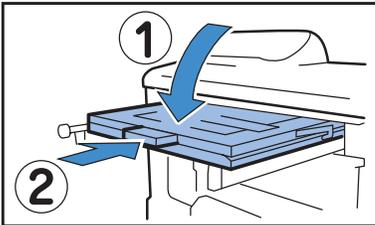
**7 Return the tab at the left of the Reversing Path Cover to its original position.**
