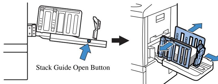
When removing printed paper from the Paper Receiving Tray, press this button to spread the Stack Guides for easy removal.
