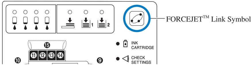
If colour management cannot be performed properly because, for example, an ink cartridge is not set, the FORCEJET™ Link Symbol goes out. At this time, check the status of consumables and settings.
