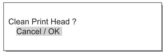
When message "Cleaning Print Head-K" blinks, cleaning is performed. After cleaning is complete, the screen in step 4 will appear again.
