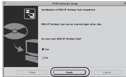
The RISO IP Setting Tool is installed. Next specify the IP address for the controller. Selecting **[Yes]** starts the RISO IP Setting Tool, so perform the operations starting with step 2 under “Network Settings” p.20.
