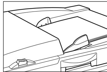
The ADF unit detects the document, and automatically opens the Master Making Basic Screen
