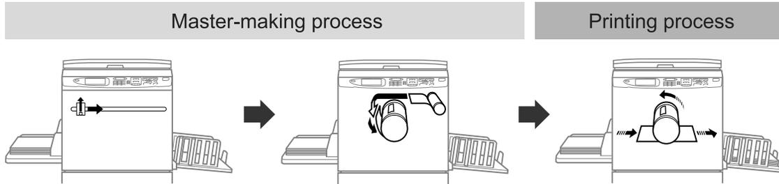
A placed original is scanned by the scanner, and a generated master is rolled around the Print Cylinder (Drum). After a while, proof copy is performed. After checking the print result, enter the number of copies to be printed and start printing.
