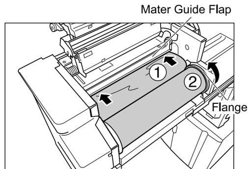
Insert the leading edge of the master into its entrance under the Master Guide Flap and advance it as far in as it will go ( ① ). If the Master is loose, turn the flange at the right towards the rear and rewind ( ② ).
