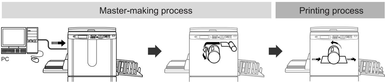
Data sent from a computer is transformed into images, and a generated master is rolled around the Print Cylinder (Drum). You can send instructions for printing from the computer (through the printer driver).
