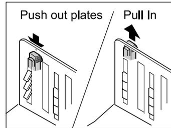
Alignment of paper is affected by sizes and strength of paper. Adjust the Paper Arrangers so that printed paper is aligned. Press the Paper Arranger to push the plates out, pull up to pull them in.
