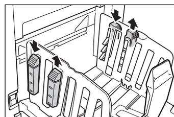
Press to open the two Paper Arrangers (right and left) closer to the machine.
