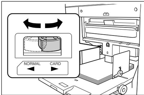
Position the Paper Feed Pressure Adjustment Lever according to the finish of the paper.
