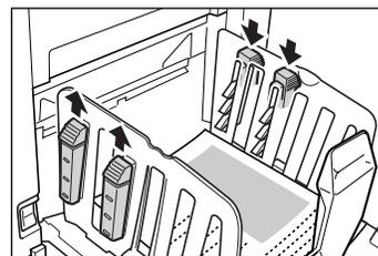
Press to open the two Paper Arrangers on the more heavily printed side.
