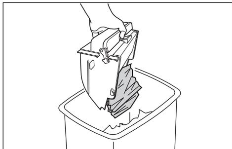
Tilt the Master Disposal Box down and discard the used masters.
