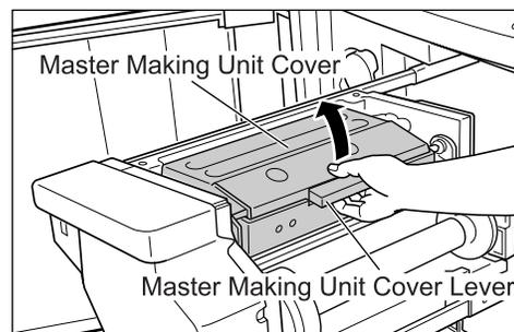
Grasp the Master Making Unit Cover Lever and open the Master Making Unit Cover.
