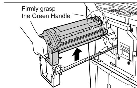
Use both hands to lift the Print Cylinder (Drum) straight up to remove from the rail. Proceed with replacing the cylinder (drum), removing the paper jam, etc..
