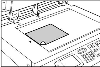
Place the original face down on Stage Glass. Align center on the top edge, and close Stage Cover.
