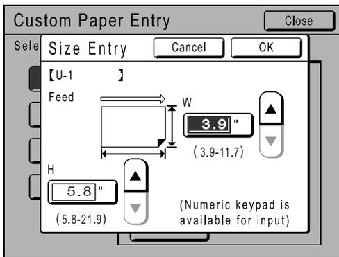
Facing towards the paper feeding direction (into Paper Feed Tray), enter W (width) and H (height). Touch either , or use Print Quantity Keys.
