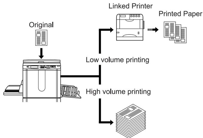
Automatically select an output device based on number of copies when printing from a computer. (When Online Auto-Link is enabled)
