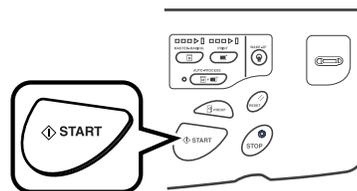
Starts scanning of the original. A master is made once the scan is completed, and a proof copy will be printed.
