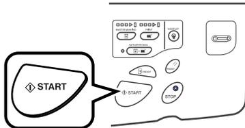
The master is made and copies printed in accordance with the Job Memory setting.
