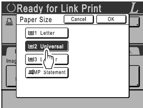
2) Touch the button corresponding to the size of the paper loaded in the "Universal" tray.
