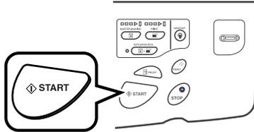
The scan of the original begins. The scanned original data is sent to the Linked Printer, and the specified number of copies is printed from the Linked Printer.
