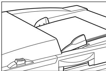
Use the ADF unit if you are printing multiple originals in succession. Place originals face-down and then adjust the ADF Original Guides to the width of the originals. Insert the originals as far into the ADF unit as possible.
