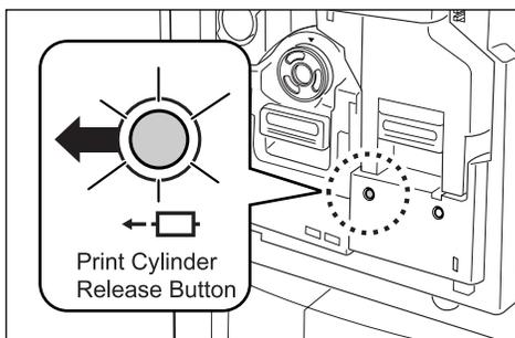
If the indicator is off, press the Print Cylinder (Drum) Release Button to turn it on.
