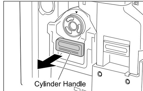
Grasp the Print Cylinder (Drum) Handle and slowly pull until the Print Cylinder (Drum) is completely extended.
