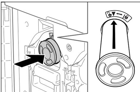
Align the arrow on the Ink Cartridge to the ▼ mark on the cylinder (drum) unit, and insert until it stops.
