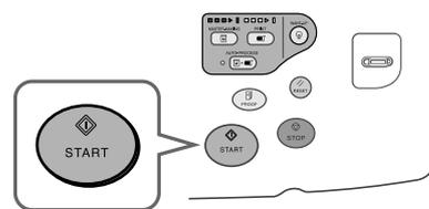
The scan of the original for Cylinder (Drum) 1 begins. Once the scan has completed, the master is made for Cylinder (Drum) 1.
