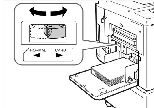
Position the Paper Feed Pressure Adjustment Lever according to the finish of the paper.
