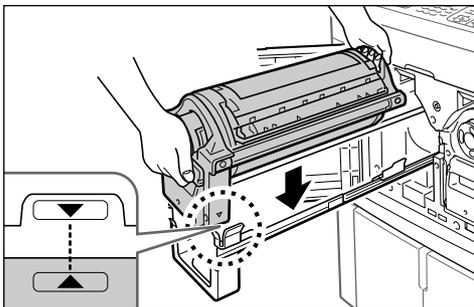
Align the ▼ mark on the Print Cylinder (Drum) with the ▲ mark on the guide, and place the Print Cylinder (Drum) horizontally onto the guide.
