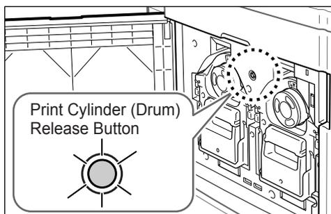
If the indicator is off, press the Print Cylinder (Drum) Release Button to turn it on.
