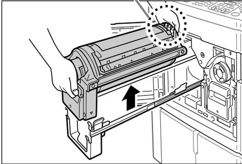
Use both hands to lift the Print Cylinder (Drum) straight up to remove from the rail. Proceed with replacing the cylinder (drum), removing the paper jam, etc..
