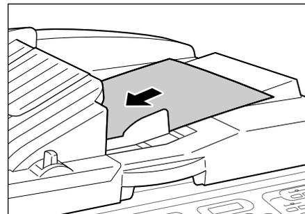
Use the ADF unit if you are printing multiple originals in succession. Place originals face-down and then adjust the ADF Original Guides to the width of the originals. Insert the originals as far into the ADF unit as possible.
