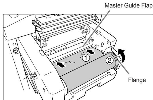
Insert the leading edge of the master into its entrance under the Master Guide Flap and advance it as far in as it will go ( ① ). If the Master is loose, turn the flange at the right towards the rear and rewind ( ② ).
