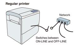
A regular printer's ON-LINE/OFF-LINE switches between the Network and the Print Controller. Therefore, data cannot be sent to the printer while the machine is OFF-LINE.
