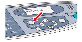
Press the  $\triangle$  or  $\overline{\bigtriangledown}$  key to display "Configuration", and then press the [OK] Key.
