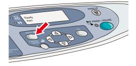
When the display shows [Temp Data Retrieve], confirm with the [OK] Key.
