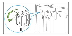
2 Similarly lift the back corrugator while pressing it toward the machine (to the left).
