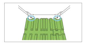
2 Set the carriage by inserting its protrusions into the holes in the stacking tray.
