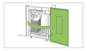
3 Pull out the carriage along with the stacking tray on it.
