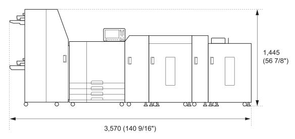
The width is 3,760 (148 1/32") when covers and operation parts are open.
