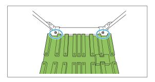
Set the carriage by inserting its protrusions into the holes in the stacking tray.
