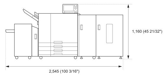
The width is 2,555 mm (100 19/32") when covers and operation parts are open.
