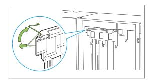
2 Similarly lift the back corrugator while pressing it toward the machine (to the left).
