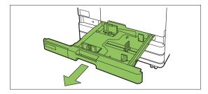
Hold the lever of the paper feed guide, and pull it forward to spread the paper feed guide until it stops.
