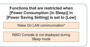
\* Windows: Set in the [Environment] tab on the printer driver. Mac OS: Set in the [Utility] tab on the printer driver.
