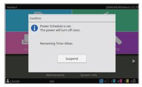
If you do not want the machine to turn off, touch [Suspend]. Close the [Confirm] screen to suspend the power-off process. The [Confirm] screen will be displayed again after one minute.
