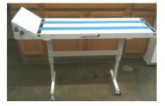
Step 9. Loosen the locking levers on both stand legs to adjust the conveyor height. It is generally easier to adjust one end at a time and lock in place while adjusting the other end.
