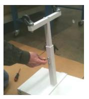
Step 7. Using the 1/2" long button head screws and lock washers, attach the cross bar to the stand legs. After complete assembly, tighten all bolts completely.
