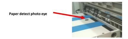
The conveyor also features a "continuous run" switch on the back plate. When in the down position, this switch causes the conveyor to run continuously and disables the paper detect photo eye. When using longer documents or documents that the photo eye has trouble detecting, continuous run mode can help
