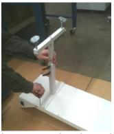
Step 5. Attach the stand leg with the casters to the other end of the conveyor as shown.
