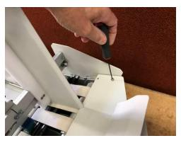
Step 14. Center the top plate between the feeder side plates so that it does not rub either side and then tighten all four screws
