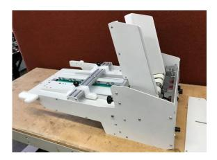
Step 10. Using a 3/32" Allen wrench, remove the four button head screws from the top plate supports as shown. Be careful to avoid dropping these screws into the feeder.
