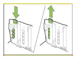
Normally, the paper arrangers should be extended when printing on paper that is B4 (10x14-inch) size or smaller. How paper is stacked after printing varies depending on stiffness and other factors. Adjust the paper arrangers as needed.
