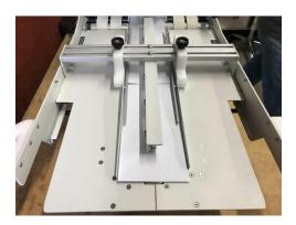
IT IS A GOOD IDEA TO TEST THE FEEDER FOR SEVERAL ENVELOPES AGAIN AFTER TIGHTENING THE GUIDES TO ENSURE CONSISTENT ENVELOPE MOVEMENT.
