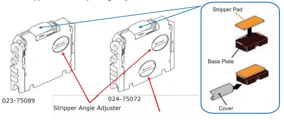
2- Adjust the Paper Feed Pressure as shown below:
