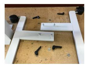
NOTE: The stand legs feature two casters each. The casters with the lock will be on the same side of the stand as the stand cross bar
