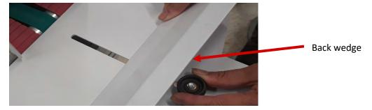
Step 4. Rotate the separator adjustment knob on top of the separator assembly clockwise several turns to raise the separator tip
