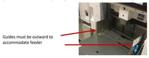
Step 23. Carefully position the feeder in front of the printer feed tray parallel with the tray
