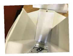
Step 8. Push the envelope forward toward the acceleration table until the leading edge is under the separator tip as shown here:
