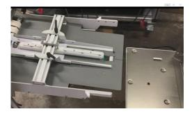
The feeder acceleration table (delivery table) is equipped with supports (shown below) that will rest on the printer feed tray. When the stand height is set correctly, these supports should slide onto the printer's tray as the feeder is moved into position. (With the tray all the way down) During operation, the printer tray will lift the acceleration table of the feeder to the proper height.
