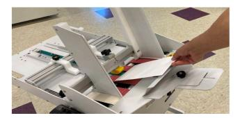
Step 6. Rotate the paper guide adjustment knob to move the paper guides inward towards the envelope.
