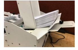
Step 13. Loosen the locking knobs on the acceleration table paper guides and slide them into position so the leading edge of the envelope under the separator will enter the acceleration table between the paper guides
