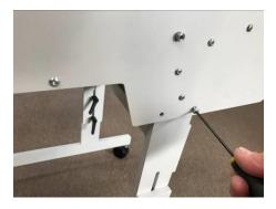
Step 18. After all four bolts are installed, hold the feeder level and tighten the bolts.
