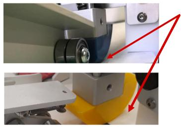
Lead edge of envelope should buckle downward between the white feed belts but not be pinched against the green belt
