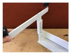
Step 5. Place a flat washer on the top bolt and then thread one of the locking levers on to the bolt
