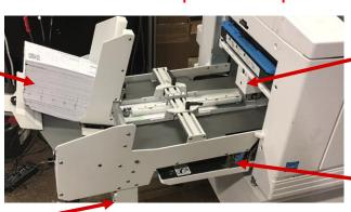
Feeder advances envelope into position under the printers feed roller
