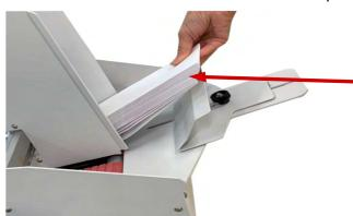
"Shingling" the small stack of envelopes before placing them in the hopper will help the lead edge of the stack conform to the curvature of the paper guides and separator tip
