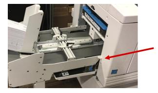
Step 28. Set the feeder speed dial at approximately 50% (12:00) and switch power to the feeder on. The feeder should advance the first envelope up to the printer and under the printer's feed roller.
