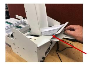
The back wedge should lift the trailing edge of the envelopes off of the top plate and feed belts.
