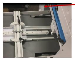
Postion block. Should slide between printer side plates closely
