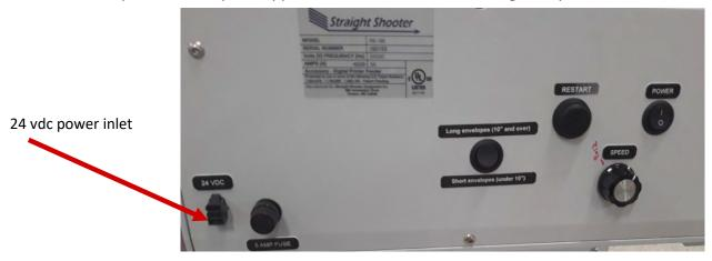
Step 15. Turn the speed adjust dial counterclockwise to set the feeder at a moderate (slow) speed.
