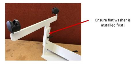
Step 6. Raise the leg assembly so the top locking lever screw is all the way up in the slot and then tighten the locking lever. Then install a washer and locking lever on the lower bolt.
