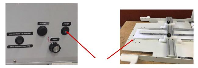
When power is switched on, the bottom envelope should advance to the stop sensor positioned near the end of the acceleration table.
