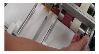
Step 7. Position the paper guides close to the edges of your envelope. The paper guides are self-centering, so allow them to move the envelope a bit if necessary. Ensure that the guides are not too tight against the envelope. A small gap between the guides and the envelope edges is suitable.
