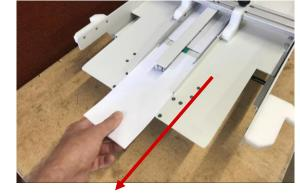
Step 19. Repeat this test to feed and remove envelopes approximately 5 to 10 times. As you pull each envelope away, observe the advance of the subsequent envelopes. Each envelope should follow the prior envelope closely as they advance down the acceleration table.
