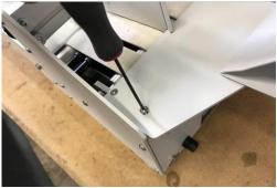
Step 13. Install the two button head screws in the other end of the top plate
