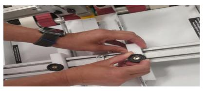
It is a good idea to keep these paper guides a little bit wide for now, so they do not restrict the envelope movement. These can be fine-tuned later once envelopes are advanced into the acceleration table
