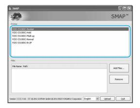
On the printer list, the printer drivers installed in your computer are displayed. When installed in the standard way, the printer driver for the IS1000C / IS950C is displayed in the form of "RIP name" - "Queue".
