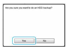
Backup begins and the print controller DATA lamp blinks. Once backup has finished, the print controller will perform the operation set for [Action after backup].
