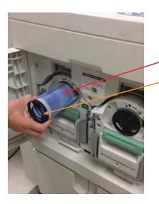
3. Pull out the ink cartridge and recycle.
