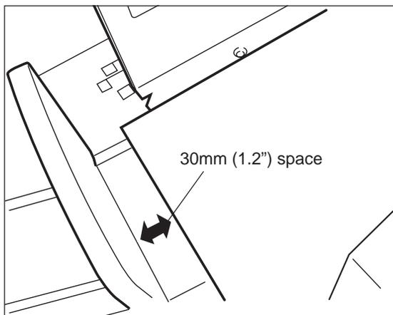
If the sheet size is smaller than B5 (or 7.2" × 10.2"), attach the Extension Stopper (accessory) to the Paper Stopper before position adjustment.
