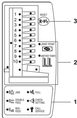
The Check & Error Display ( 1 ) indicates the current machine condition, while the Machine Monitor Display ( 2 ) shows the locations to be checked in relation with the current machine condition. The related advice message, appears in the Main Display to help you check the machine status.
