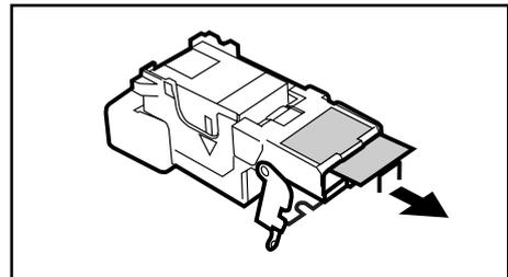
**4** Turn back the mouth tip of the staple cartridge to the initial position.
