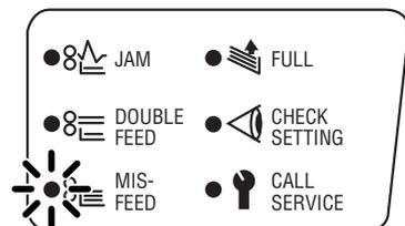
**Cause** No sheet has fed in the bin(s) indicated in the Machine Monitor Display.
