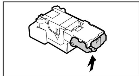
**5** Return the staple cartridge into the stapler, and close the Staple Cartridge Door.
