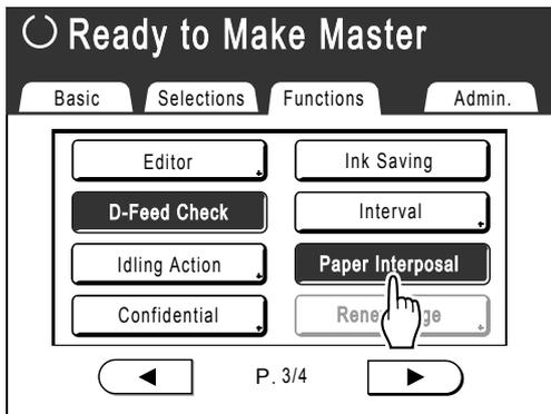
“Paper Interposal” setting is completed and the machine is ready to print.
