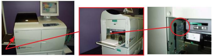
Drop the Paper Feed Tray down. Looking at the Paper Feed Tray, Serial Number is on the frame to the left to the right.
