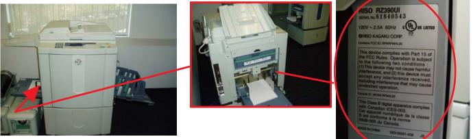
Drop the Paper Feed Tray down. Looking at the Paper Feed Tray Serial Number is on the frame to the right.
