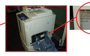
Looking at the Paper Receive Tray, Serial Number is on the frame to the right by the Power Cord.
