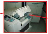
Lift the Master Making Cover. Serial Number is on the Rear Frame just above the Master Roll.
