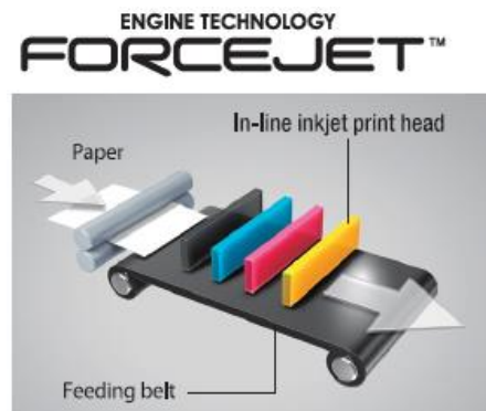
Figure 4: RISO FORCEJET Heatless Printing Technology
