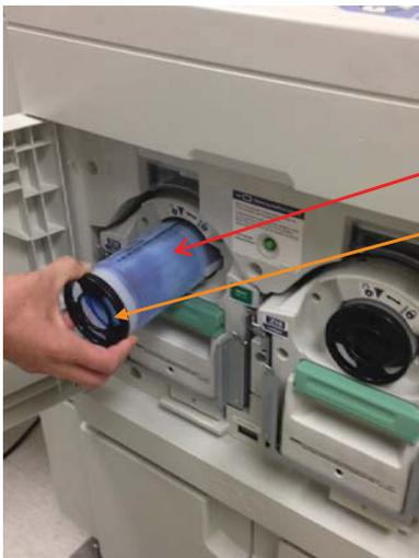
3. Pull out the ink cartridge and recycle.
