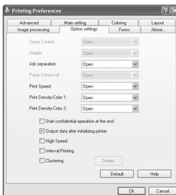
Job separation for the optional sorter and stapler, density and speed for printing, clustering and other functions can be set.
