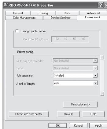
The controller IP address can be set and the device configuration confirmed.
