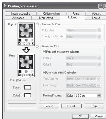
Ink colors printed, Print cylinder (drum) and coloring conditions can be set.
