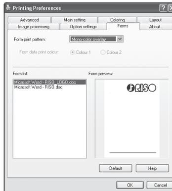
Forms registered in the printer can be combined with output data and printed.
